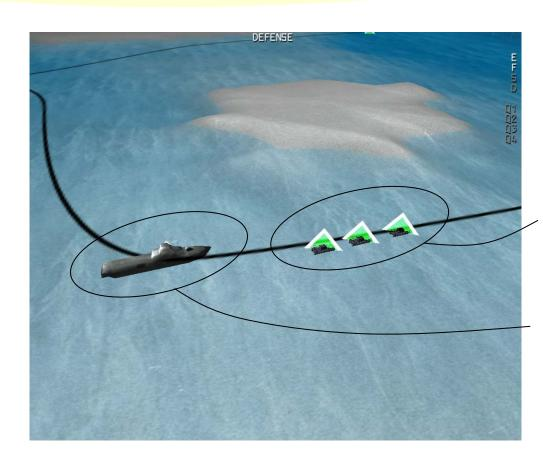
A group of self-propelled autonomous mine-sweepers (SAMs) have been activated and deployed by a transport vessel.
