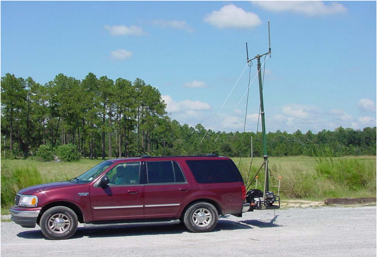
Figure 4. MSDII HMMWV/SUV used as Relay
