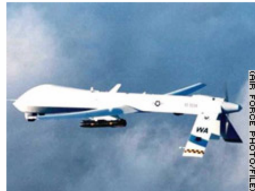
Unmanned Predator armed with Hellfire missile photographed during 2001 test flight.
