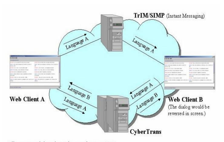
Clients are web based; can be anywhere on CFBL. Flow can also go from Client B to Client A.
