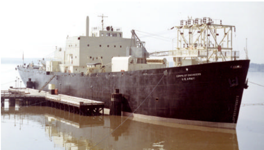
Figure 4. The MH-1A Sturgis Mobile Nuclear Power Plant Used a 45 MW Pressurized Water Reactor.
