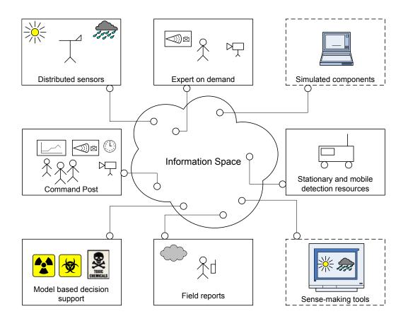
Figure 4: Overview of a test bed demonstration. The Information Space supports dynamic connection of various services such as sensors, models, experts and units. The lines in the figure between the functions and the information space illustrate communication links.
