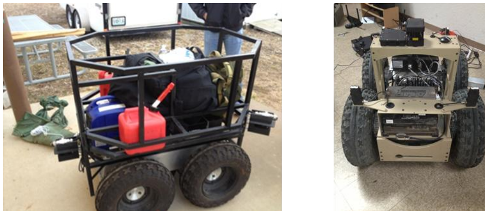
Figure 3. Segway 440X shown here at left with the Adaptive Mission Payload (AMP), a generator and 200lbs of supplies. At right is the Exponent configured Segway with UWB tags in the black cases just above and forward of the tires.
