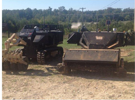
Figure 1: The ACER and Segway robots as part of a wagon train in a route clearance mission (left). The image at right shows the ACER with different configurations for route clearance (mine roller on left and mine flail on right).
