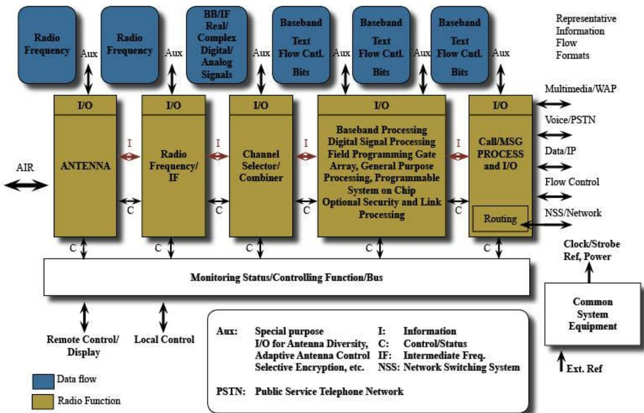
Figure 2. Notional architecture for a SDR. Adopted from (5)
