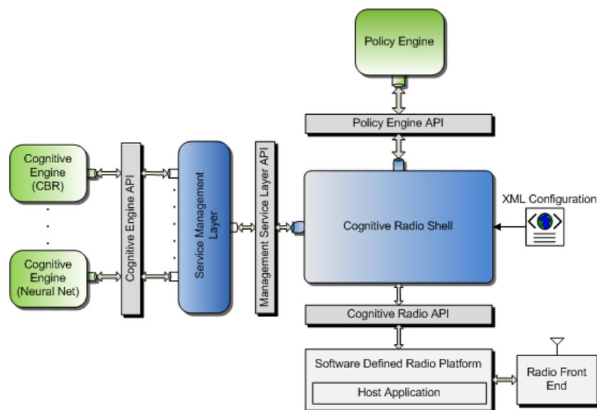
Figure 3. An example of open source Cognitive Radio architecture. Adopted from (13) cf. (14).
