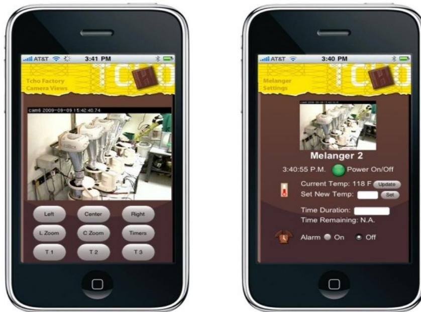
**Figure 5. Smart-phone (iPhone) based views for monitoring and controlling devices in a physical factory, from Back, Kimber, *et al.* [2010].**
