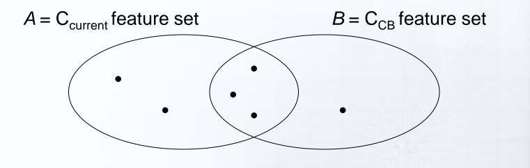
Tversky's index =  $S(A,B) = \frac{|A \cap B|}{|A \cap B| + \alpha \cdot |A - B| + \beta \cdot |B - A|}$
