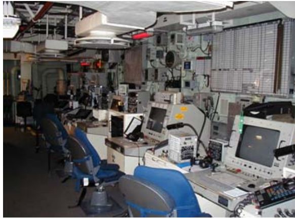
Command & Control in Submarine Control Room (VCS)
