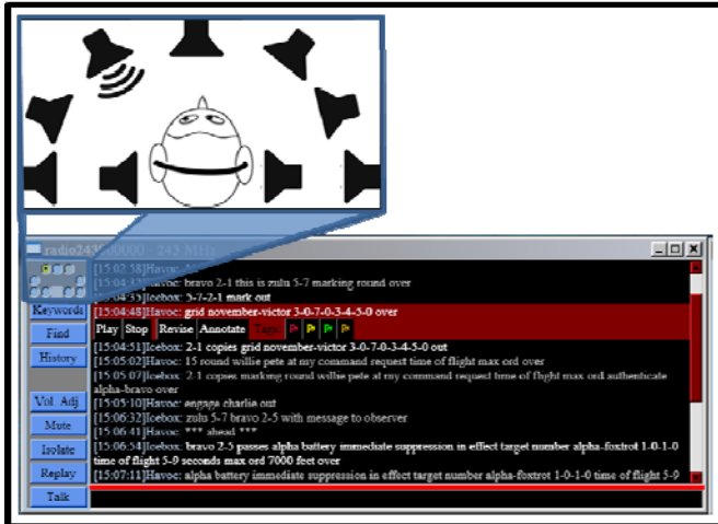
Figure 2. Representation of the virtual sound source based on selection in the Spatial Audio control. A user selects the location they wish to hear the communication to virtually originate from and the system selects the corresponding HRFT to filter the audio stream.
