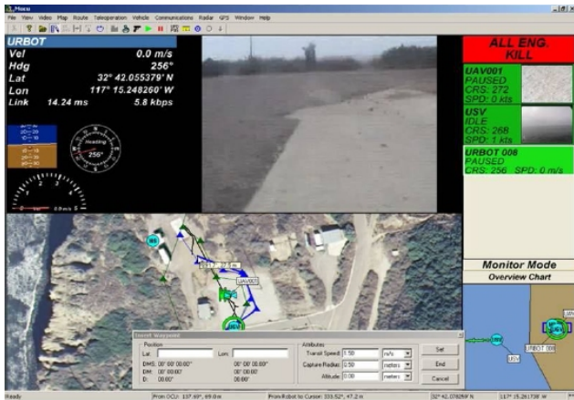
Figure 2. Screen-Shot of MOCU Configured as A Multi-Vehicle (UAV/USV/UGV) Controller with Video From A Manportable UGV. [2]
