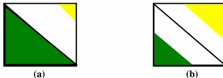
Figure 6: (a) An SCS for an alternative with the best score (full green triangle) and very little conflict (yellow triangle), and (b) An SCS for an alternative with a score only a third as good as the best score and approximately a third of its model's variable options in conflict.
