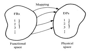
Figure 1. The Mapping From The Functional Space (Or Domain) To The Physical Space (Or Domain), [Suh 1990]. Note that the DPs in the physical space are chosen to satisfy the FRs in the functional domain.
